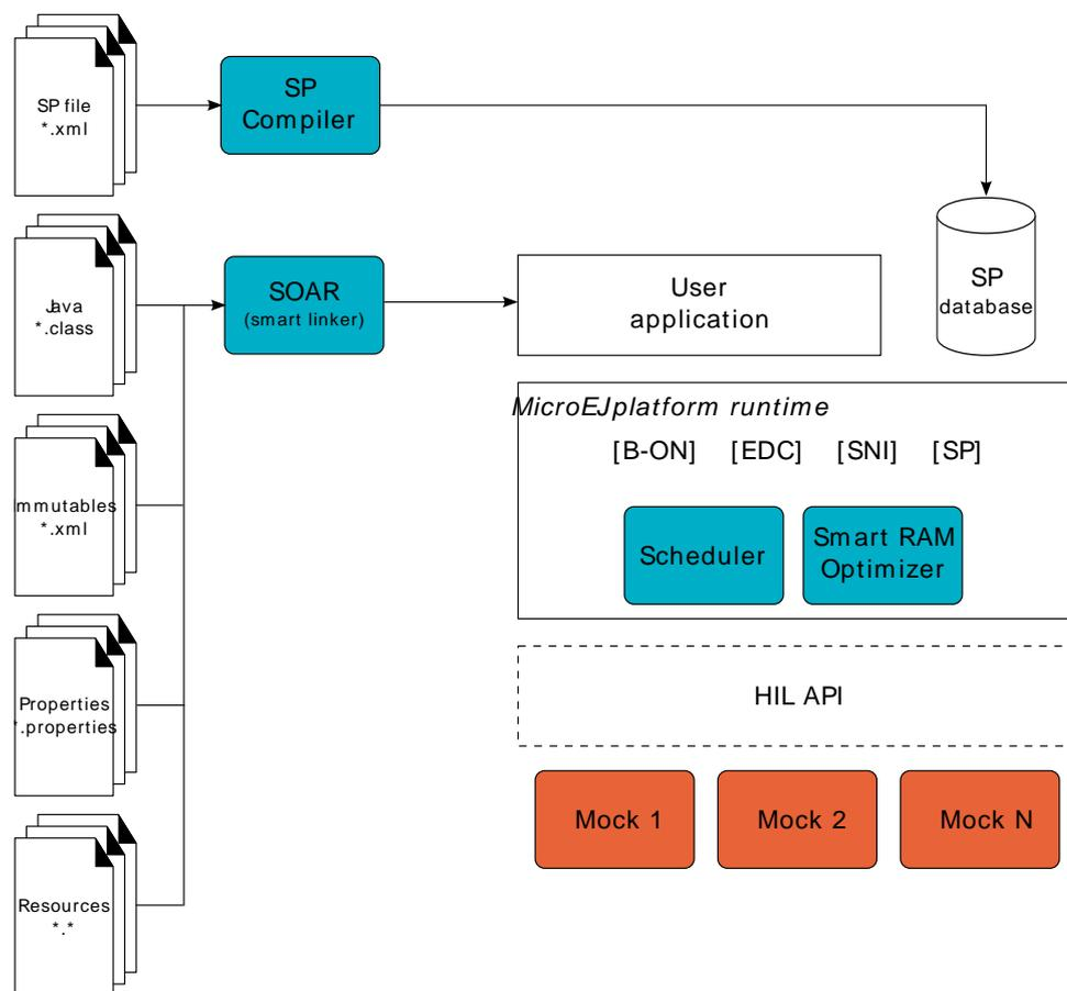
Figure 20.1. The HIL Connects the MicroEJ simulator to the Workstation.
