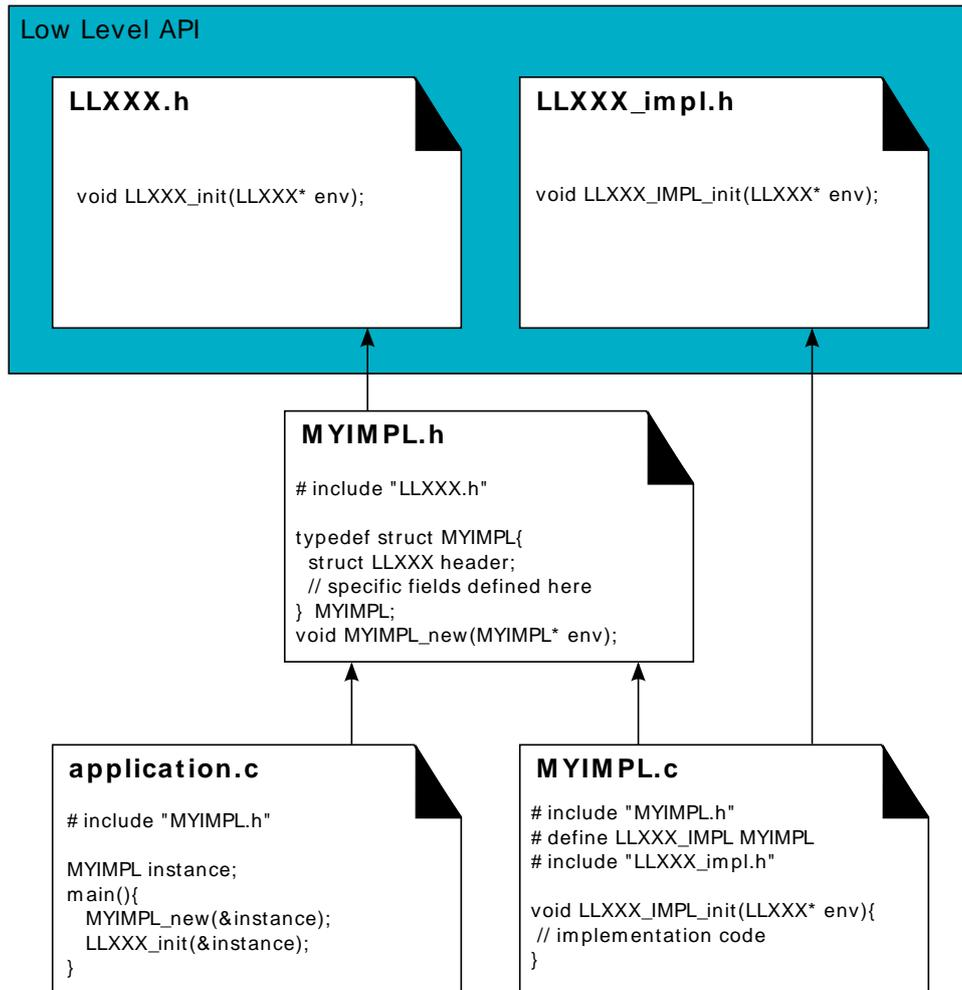
Figure 5.5. Low Level API Pattern (multiple implementations/instances)
