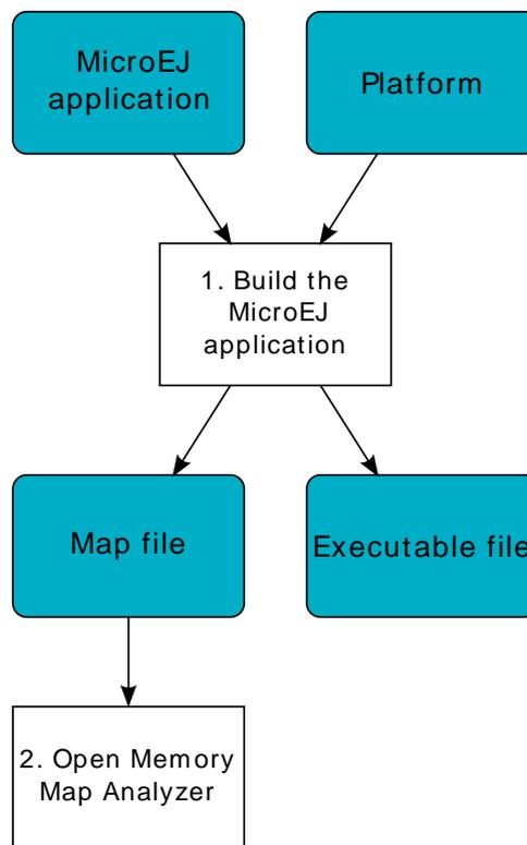
Figure 19.1. Memory Map Analyzer Process
