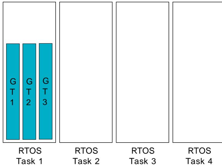
Figure 7.2. A Green Threads Architecture Example
