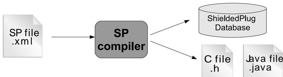
Figure 10.4. Shielded Plug Compiler Flow.
