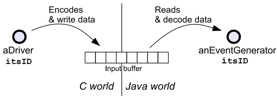
Figure 14.9. Drivers and MicroUI Event Generators Communication
