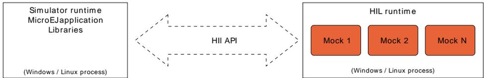
Figure 20.2. A MicroEJ simulator connected to its HIL Engine via a socket.
